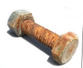
The ATF-Acetone mix was a "home brew" mix of 50-50 automatic transmission fluid and acetone. Note the "home brew" was better than any commercial product in this one particular test. Note also that "Liquid Wrench" is about as good as "Kroil" for about 20% of the price.
