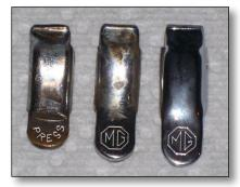
continuously through about TC6000. That means 60% of TC's should have the PRESS trigger. The transition to the "MG" logo on the trigger was a mid-TC production change, one of many subtle changes in 1948.
