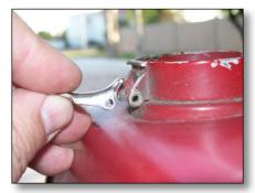
How the trigger should fit on the filler neck.
