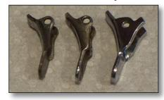
its base resulting in a needed change to the trigger. "Feet" were added to the trigger as a mechanical stop to prevent the trigger from stopping on the painted top of the tank. This has created a problem for pre-TD owners. The later trigger does not work on the TABC tank.
