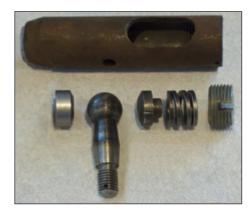
Drag Link End (DLE) - there is just one of these and the ball has a tapered shaft.
