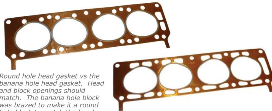
*Round hole head gasket vs the banana hole head gasket. Head and block openings should match. The banana hole block was brazed to make it a round hole block to match the head.*
