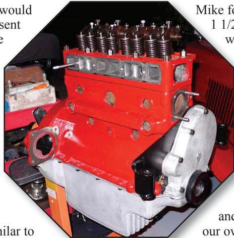
The reason for the round holes was that 1500cc head gaskets were for late TF's and only came with round holes. During the time we were waiting for the block we purchased a new crank, set of 1500cc pistons, reground TF cam and all the gaskets necessary. Mike had a restored late type large sump that I bought. Mike looked in his spare parts pile and came up with a treasure of things that we had never thought of... used original TF1500 intake and exhaust manifolds.
