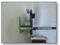
Fit new LED circuit board inside
