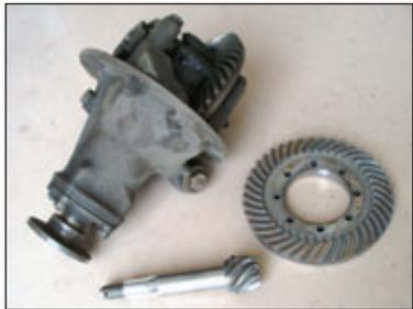
equivalent speed w/ original gearing. The benefit is added driving comfort of less noise and most importantly reduced stress on an already aged motor. There is a down side however. If you encounter hilly conditions, this gearing can create difficulty. You will have to downshift resulting in low speeds and high RPM to accomplish the same as the old gearing in rising terrain.
