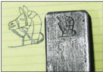
"WM" or "WML" – stamped on the pivot pin of front spring to chassis.
