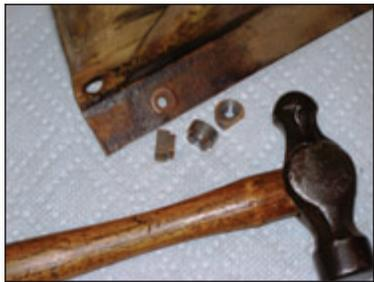
hammer, just seconds. The Double D nut is essential the same except that it has 2 flats sides. The flat sides of the holes prevents the captive nuts from turning when final install of the bolt.
