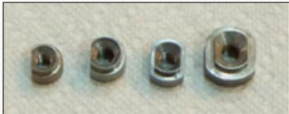
The D nut is a captive nut that gets its name from the shape of the hole needed to install into a panel. It has a very functional purpose. A captive nut in a sheet metal panel allows a single assembly line worker to install a panel without a helper holding a nut and spanner (wrench) under the car. The D nut is machined so that it has a D shaped flange that goes into the hole and then the flange is swaged to lock the nut into position. It is an easy install with a peen
