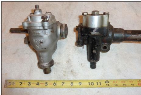
This shows the VW box on the left and original TC box on the right. VW box is very slightly larger.
