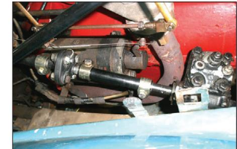
7/8" OD tube is slightly larger than the inside diameter of the VW clamp so it will be necessary to use a Dremel tool to grind a little from the diameters.
