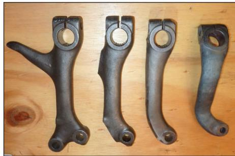
Original VW pitman arm on left, and steps to the modified arm on the right
