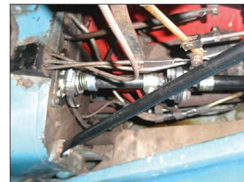
worm shaft rotates freely from lock to lock. Now snug down the 4 bolts and recheck that the input worm shaft still rotates freely. Readjust the top slotted shaft if any binding is noted. Tighten the jam nut around the top slotted shaft.
