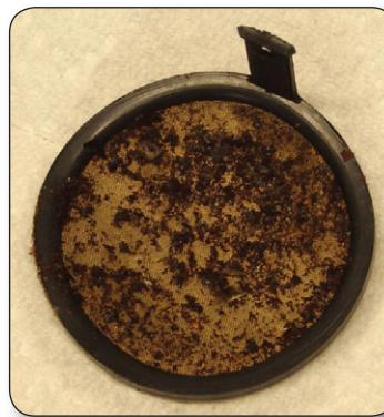
Before re-using that gas, I poured it from one gas can to another several times using a funnel with a filter. I was amazed to find just how much crud there was in the fuel. (See photo below)
