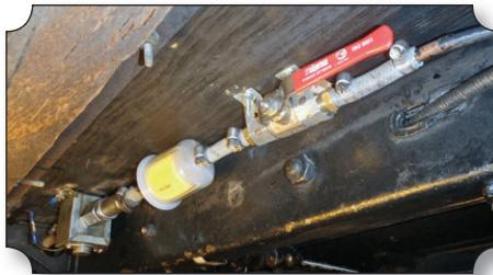
Of course, I had just filled the tank in Lompoc before we had given up at Vandenberg, so I had to deal with nearly ten gallons of fuel before I could do anything. I disconnected the fuel line at the carburetor and put a piece of 5/8 inch hose over the end, turned the ignition on to run the fuel pump and fed it into a proper gas can.
