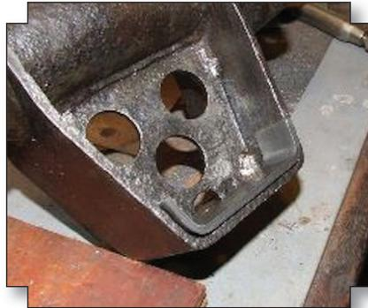
*One way of strengthening is to add material and then weld it in. Top photo shows loose piece formed and in place. Photo below shows it welded in place.*
