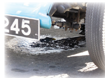
That darned water pump leak keeps getting worse but gallon jugs of water help keep the TC rolling.
