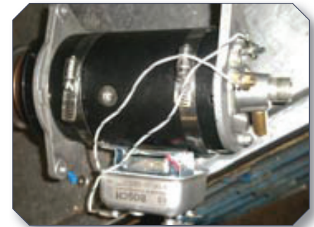
View on Bosh regulator mounted on dynamo. Held on with large hose clamps here but could be mounted elsewhere too.
