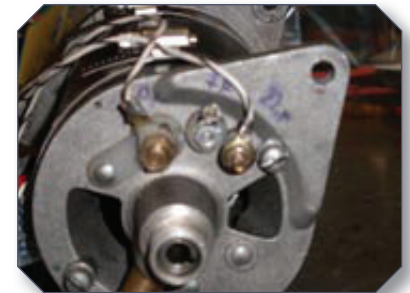
Three Terminals, IF in the middle and the one added on.
