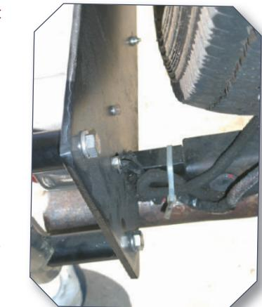
These views show the spacer blocks to the frame plus the bolts into the bumperette spacers
