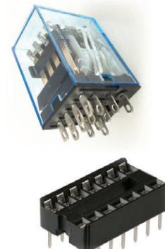
14 pin relay and the 14 pin IC socket (not all pins are used)
