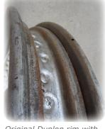
Original Dunlop rim with rolled edge and note the drain hole.
