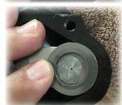
Note the black dot on the sector shaft, which is the center. Top photo with old thrust washer off center to clear casting wall. But if you move it so it is centered, then the washer overlaps the wall and does not allow adjustment
