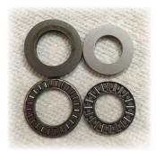
Old large bearing and washer on the left vs the newer smaller set on the right
