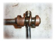
Problem: The thrust washers fit nicely into the Tompkins cover. But, due to variations in the casting of the steering box itself, the thrust washer has been found to sit on top of the box and not within the box itself and on top of the sector shaft. This means
