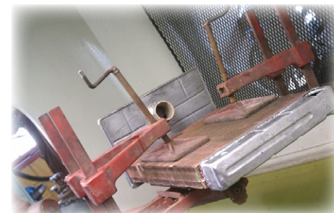
Radiator at the radiator shop being inspected, cleaned and tested
