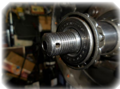
Front axle roller bearings & spacer
