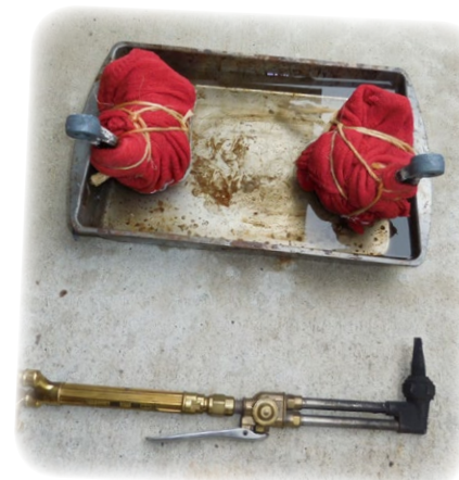
The Houdaille shocks wrapped in water bathed rags to prevent damage when annealing the lever eye holes.
