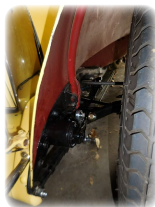
Two views of left Houdaille shock and linkage
