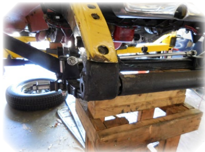
Cowl and spring pin removed
