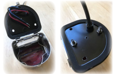
Harness through baseplate and showing the two elongated mounting holes
