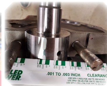
Assembling the rods and pistons on the left and checking the bearing clearance with plastigauge.
