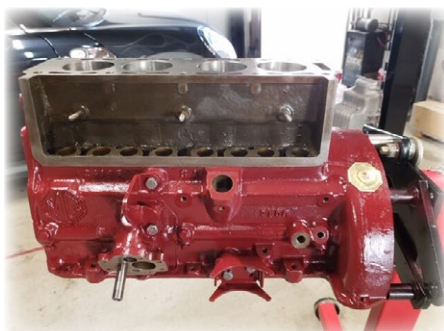
Core plugs installed on the left and painted all nice and pretty on the right.
