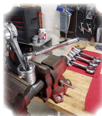
Assembling the rods and pistons on the left and checking the bearing clearance with plastigauge.
