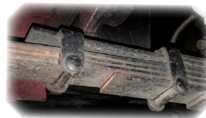
Note the rearmost shackle (left in photo) is half buried in the leaf.
