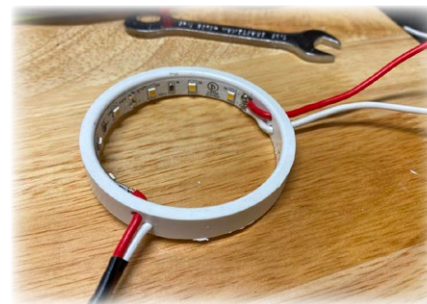
PVC ring trimmed down with LEDs
