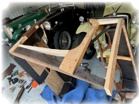
Tub needed some wood replaced so off came the metal skin and then covered back up.
