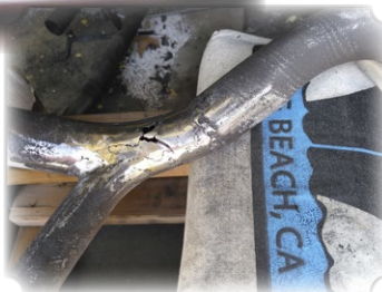
Kregg Hunsberger had a scary gremlin experience with his TC while on the way to the Conclave. Seems an old brazed connection broke on his exhaust.
