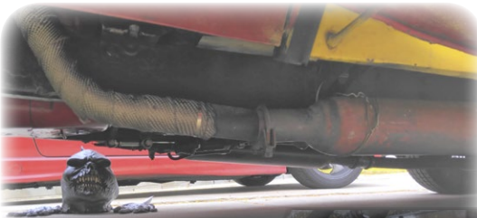
Kregg Hunsberger had a scary gremlin experience with his TC while on the way to the Conclave. Seems an old brazed connection broke on his exhaust.
