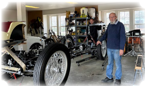
Completed chassis suspended from lifts
