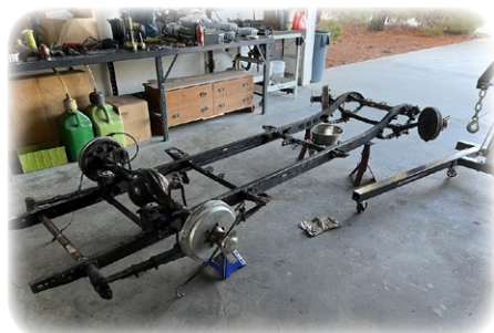
Stripping frame to powder coat
