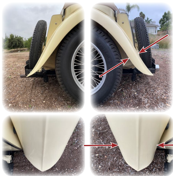
My right rear wing. Note slimmer profile towards tip as well as being wider.
