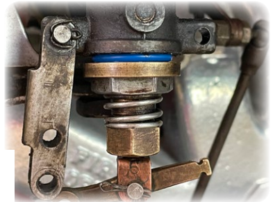
Assembly in place before final tightening. Compare to previous page when fully tightened
