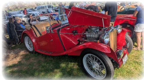
TC with a 152-cubic-inch Daimler V8 with a Weiand blower and an Edelbrock carburetor. Had issues though and barely made it off the field.
