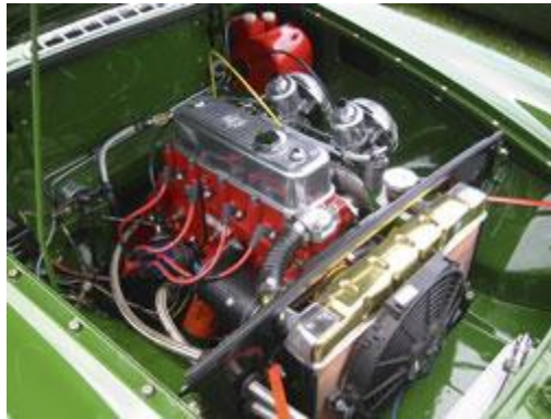
An upgraded B engine installation.....
