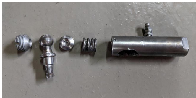
TC Track Rod End Components (L-R): Adjuster, Ball, Cup, Spring, Housing with grease fitting.
