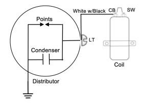
In our case the capacitor or condenser is used to protect the points by draining off
