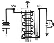
current will stop flowing and the Magnetic Field collapses. However, the collapse will induce a current impulse in the fine windings of the Secondary Coil that can, based on the number of windings, produce an output of 20,000 volts exiting the Coil through the H.T. (High Tension) and connection on the top of the Distributor.
