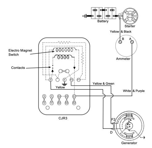
The other major function of the Cut-Out is protecting the Battery. When the Generator fails to produce enough power, either by slower speeds or failure, then the Contacts will open. If this did not happen, then power from the Battery would flow backwards through the system. From the Battery to the Starter Switch, across the Ammeter, to the CJR3 Terminal A1, then the D terminal and back to Generator and to the ground. This would result in draining the Battery.
