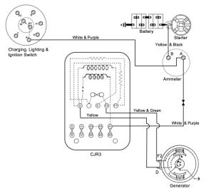
positive charging. Output from the Generator will, however, flow from Terminal A on the Ammeter and then to connection A on the CL&I Switch and on to various components by way of the IG, H and T connections.
