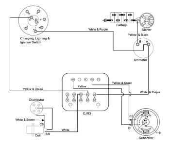
enters the Distributor Cap via its H.T. connection. From there it is sent to the sparkplugs by way of the rotor.
