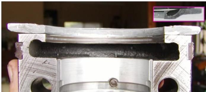
*Another view of the aluminum cover showing bottom edge after filling in front and back with JB Weld. Inset shows surface area before filling in. Wider surface would butt up against the bearing cap (not in this position though).*
