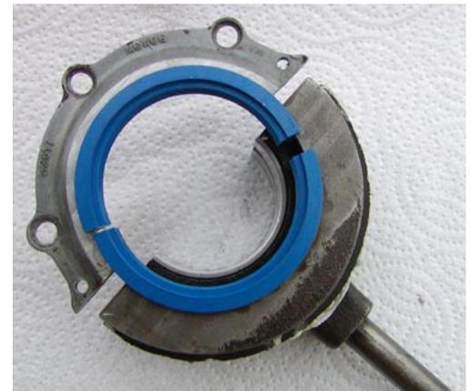
Be sure to lightly coat the seal lip with lubricant to avoid dry burn on start up.
