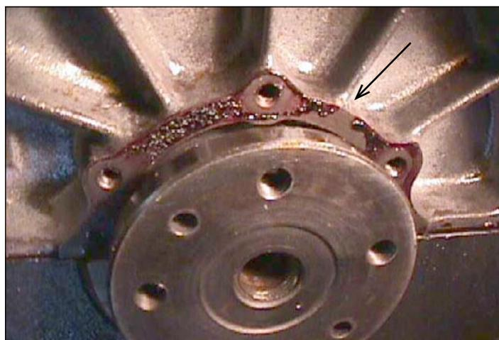
*Note gap where oil could leak past when warped cover and not enough RTV was used.*
