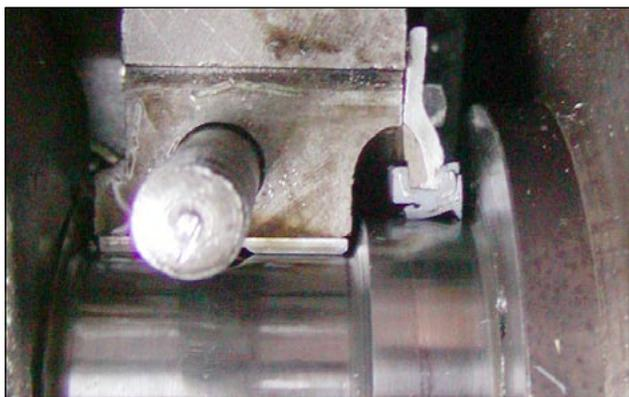
*This weld comes right up to the flange and a regular seal rides completely on it.*
