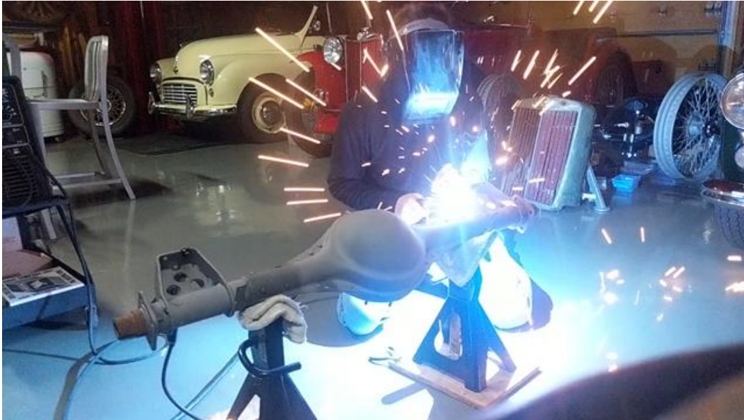
Welding cracked bolt holes. Keep a fire extinguisher handy.
