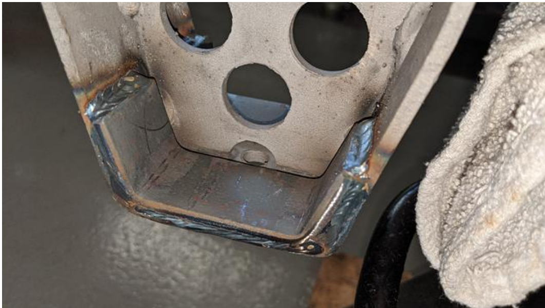
One of four gussets welded in place.
